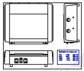
Designated a closed book laminator, it processes pass books in a closed condition. This machine was developed primarily to work with 3M Confirm film in countries that experience high humidity conditions. (Monsoon seasons) It is fitted with two (2) heater assemblies and three (3) sets of feed rollers. The first heater helps dry the book and pre-heats the laminate. The second heater stage raises the book to the required temperature to complete the lamination
